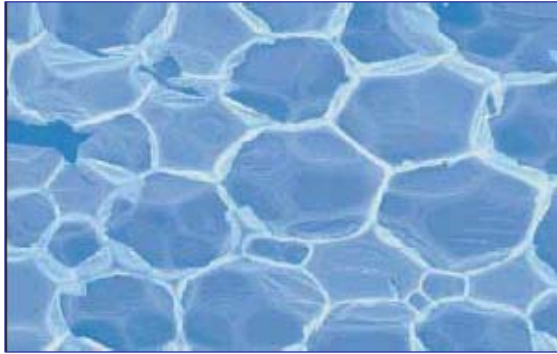
Picture 4: Cell structure of rigid polyurethane foam (PUR/PIR)
